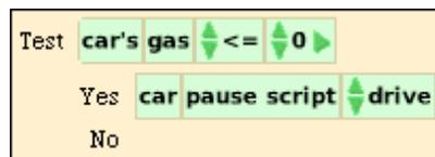
Where does the tile “car’s gas  $\leq 0$ ” come from? If you drag out the variable name “car’s gas” which you created, (*do not drag by the white arrow*), then when placed down correctly next to the TEST, it will expand to something like “car’s gas  $< 5$ ”, and at that point you can change the number you’re comparing it to, as well as whether the comparison is for less than, greater than, etc.
